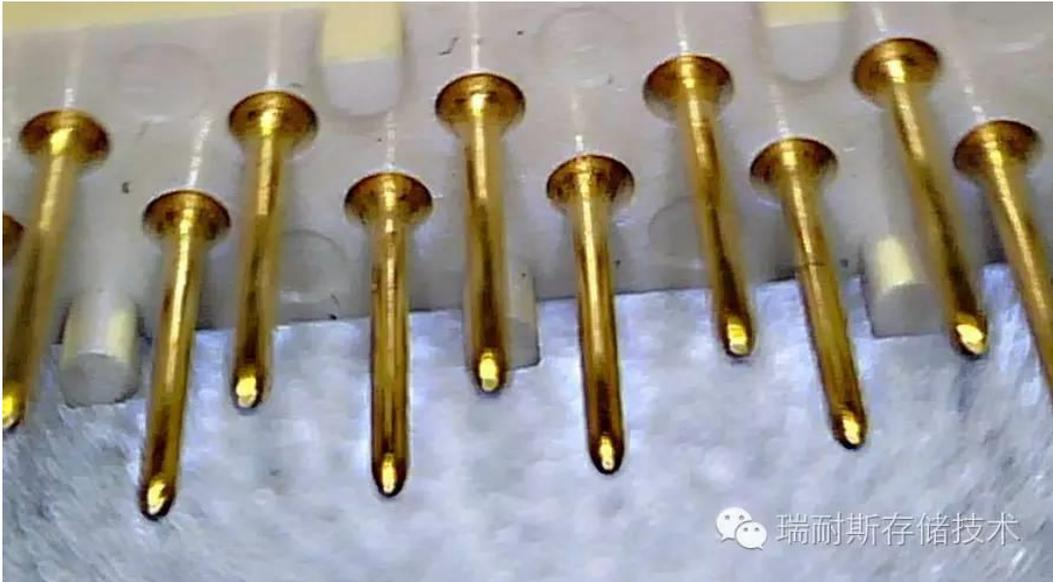
2. To be rugged, the female connector have to not just ensure easy insertion and extraction but also ensure no bad contact or damage to the tiny pins when facing intense shock & vibration, therefore the female connector is designed with pipe in pipe casing structure and hyperboloid contact technology, providing buffer allowance and meanwhile avoiding bad contact against the vibration of the male connector in any direction through the elastic pins on 5 angles.
